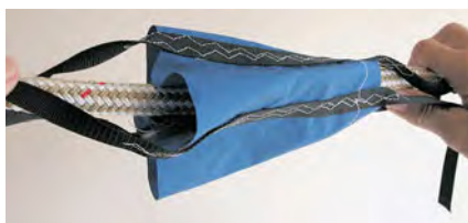
Cone configuration and bridle arrangement for a Jordan series drogue. A 30,000 lb. boat needs 300 feet of \frac{3}{4} " nylon line and 132 cones.
